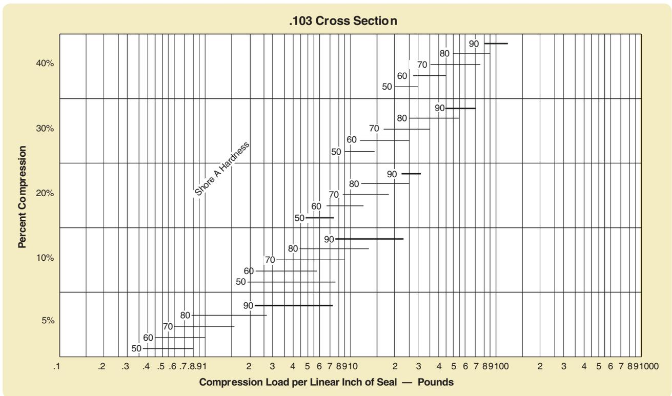
Figure 2-5: .103 Cross Section
