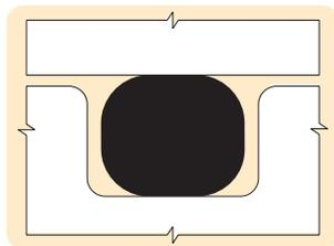
Figure 1-4: O-Ring Installed
