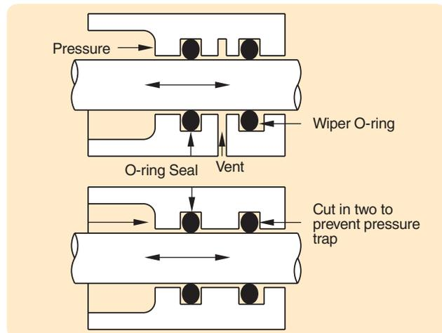
Figure 1-14: Wiper Installation
