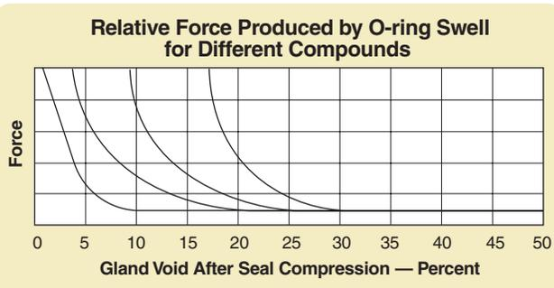
Figure 2-20: Relative Force Produced by O-ring Swell
