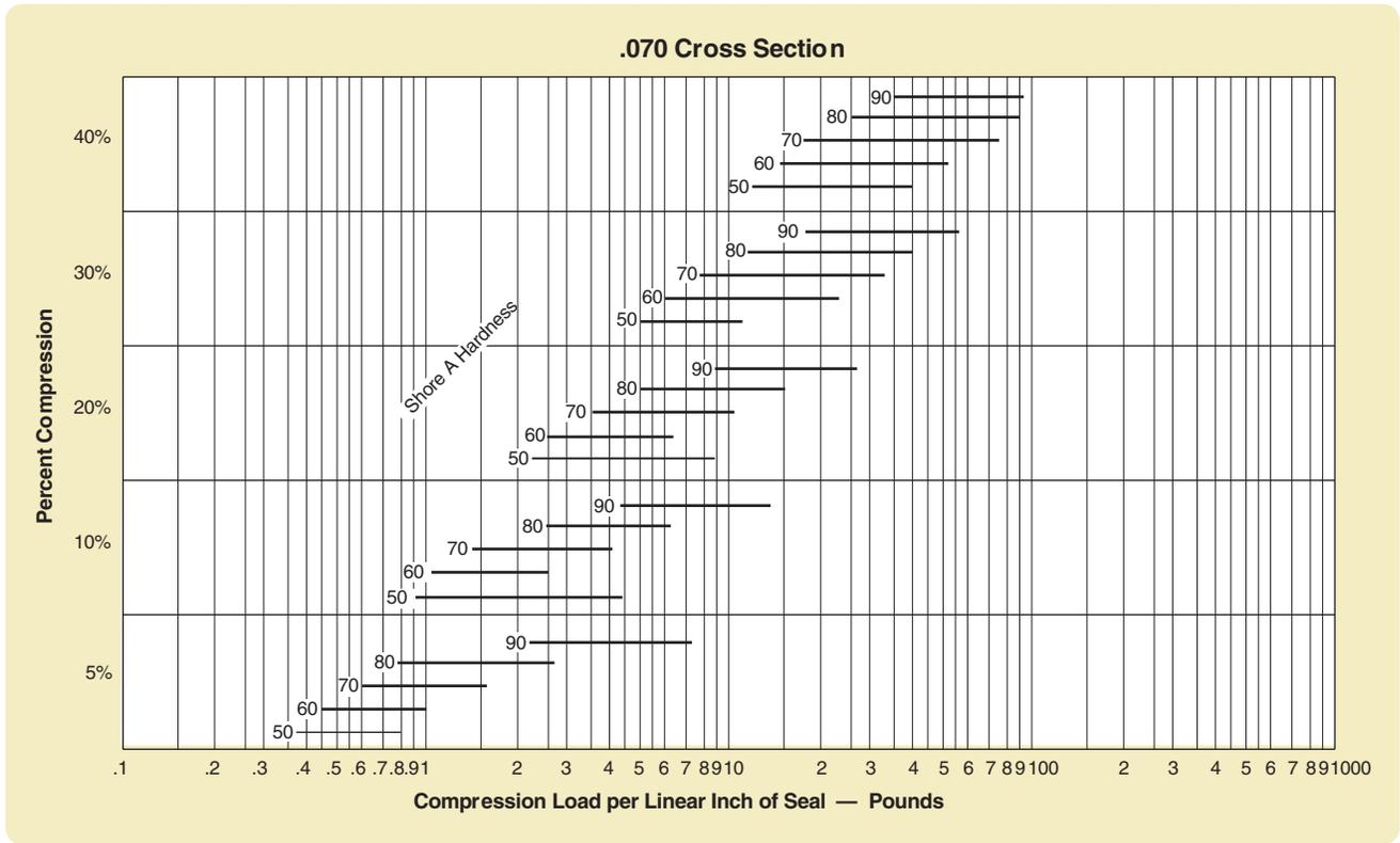
Figure 2-4: .070 Cross Section
