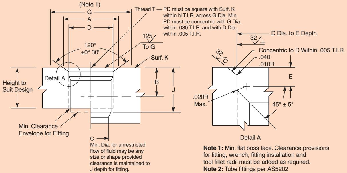
**Boss Dimensions for Military Straight Thread Tube Fitting O-ring Gaskets per AS5202 (Supersedes AND10049, AND10050 and MS33649)**
