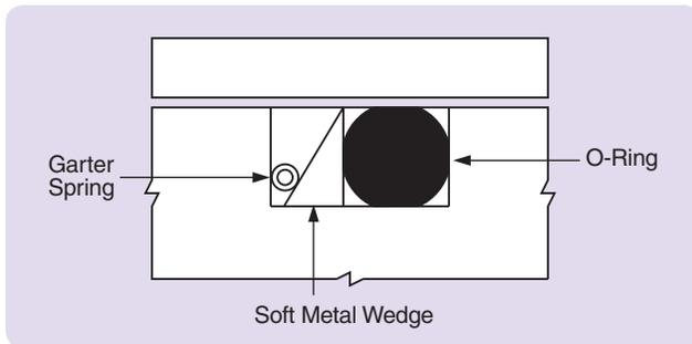
Figure 3-1: Spring-Loading for Low Temperature
