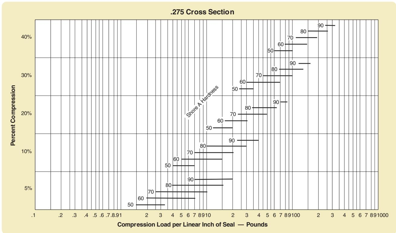
Figure 2-8: .275 Cross Section
