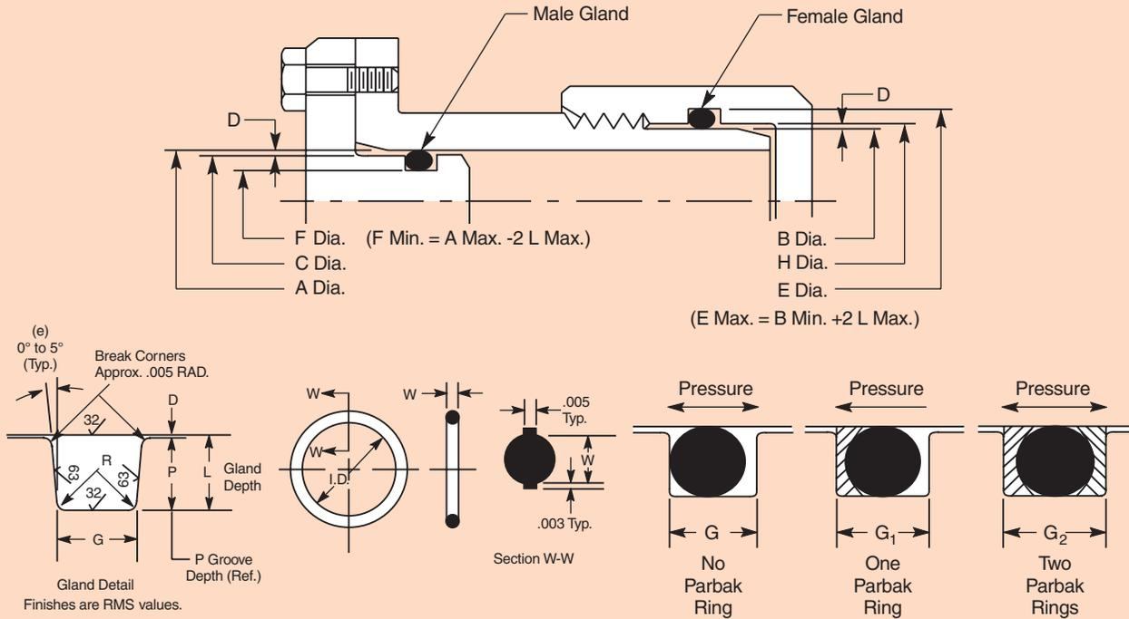
**Gland Design, O-Ring and Other Elastomeric Seals (SAE AS5857)**
