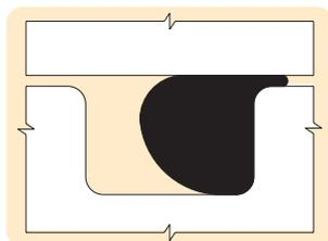
Figure 1-6: O-Ring Extruding
