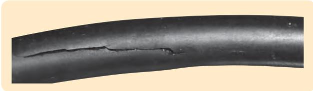
Figure 10-4: O-Ring Damaged by Explosive Decompression
