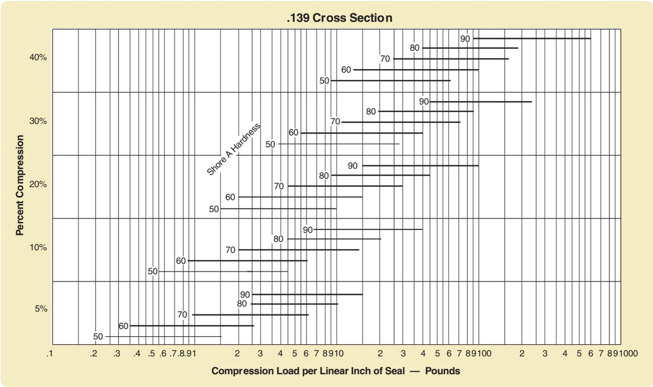
Figure 2-6: .139 Cross Section
