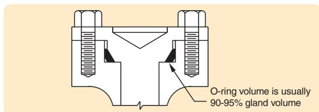
Figure 1-13: Crush Installation
