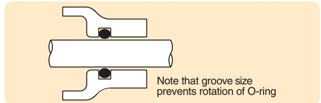
Figure 1-11: Rotary Seal
