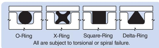
Figure 5-17: Ring Cross-Sections for Reciprocating Seals
