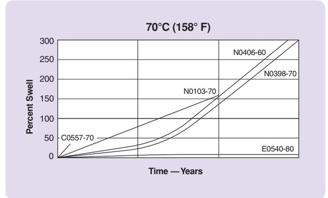
Figure 3-13: Water and Steam Resistance at 70°C (158°F)
