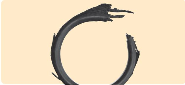
Figure 10-2: Extruded O-Ring
