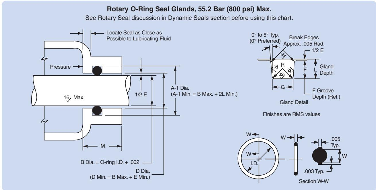
**Note:** Due to effect of centrifugal force, do not locate groove in shaft. Refer to Design Chart 5-4 (below) and Design Table 5-4 for dimensions.
