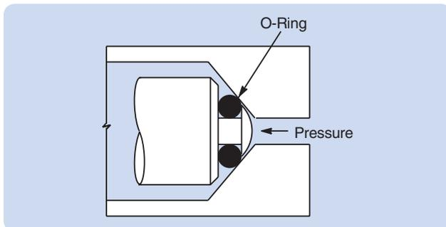
Figure 5-22: Valve Seat Seal, Standard Groove
