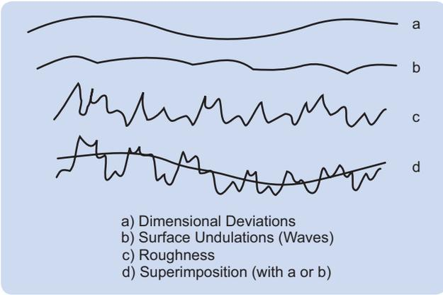
Figure 5-3: Surface Finish Structure
